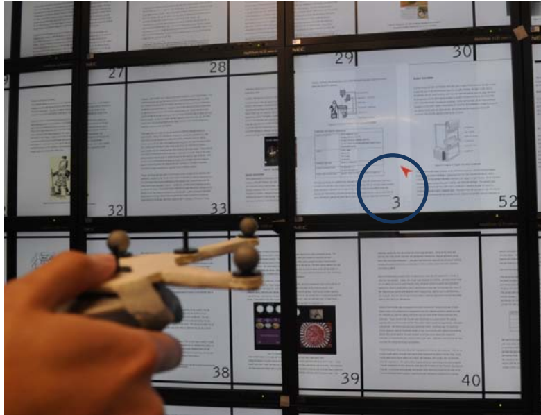
Figure 2. A user juxtaposes two pages to compare figures using handheld interface. Its red pointer is shown inside a circle.
